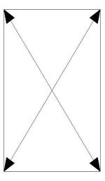
2. Using a tape measure, check the rough opening. Measure diagonally across the opening. Diagonal measurements need be equal within ¼".
